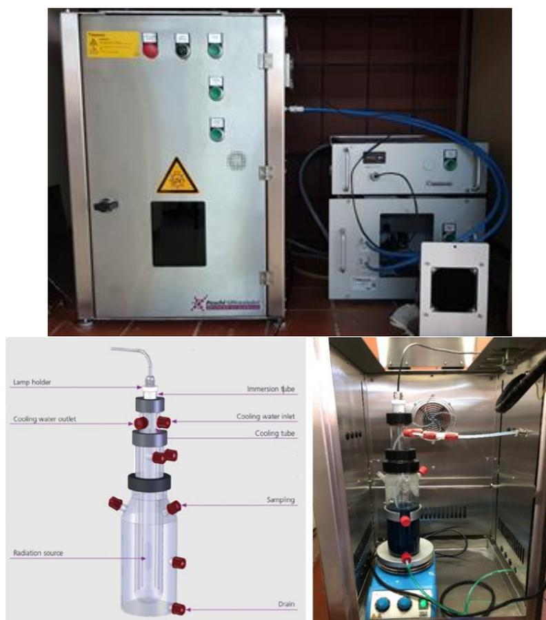
**Figure 2.** Photoreactor set up by Peschl Ultraviolet GmbH, Mainz -Germany.
