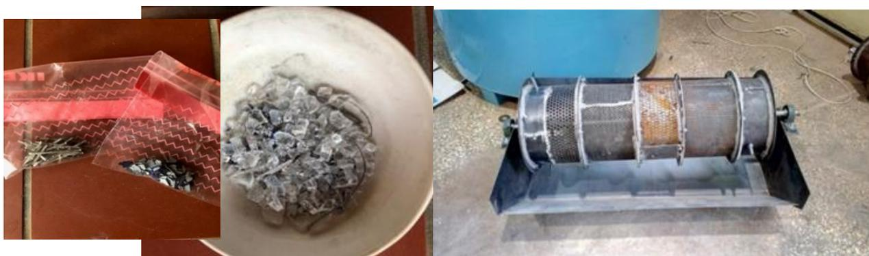
**Figure 1.** Silicon flakes, glass and electrodes separated after thermal treatment
